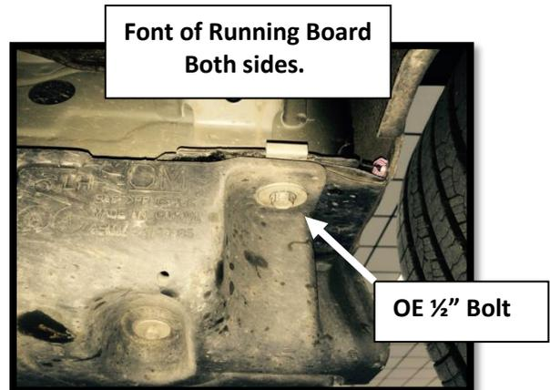
**Step 2:** Repeat step one with passenger side. **NOTE** . Be careful not to damage AC lines when removing factory running board. **Fig. B**
