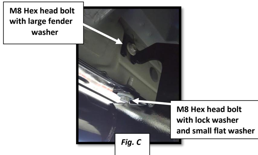
**Step 4:** Insert the supplied M8 x 1.25 Hex head bolt and M10 x 30 Fender washer into the bracket and upper threaded hole. Leave loose at this time. **Fig. C**
